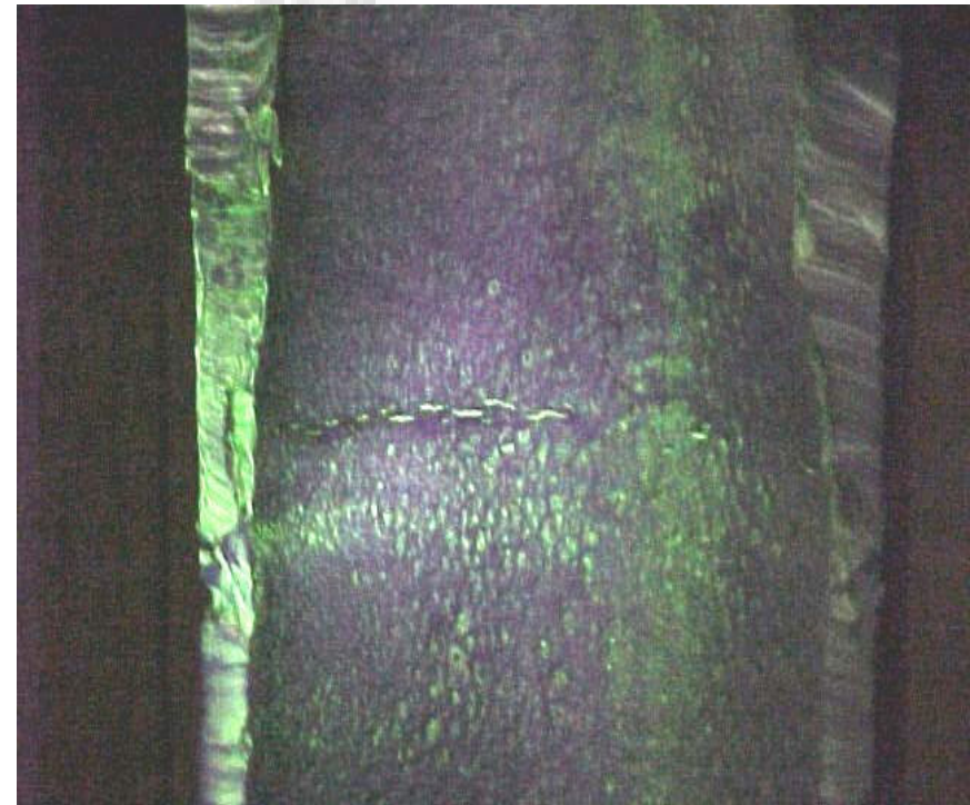
Wet Fluorescent MPI Fatigue Cracking
